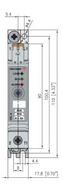
Housing width tolerance +0.5mm, -0mm as per DIN 43880. All other tolerances +/- 0.5mm. Dimensions in mm.
