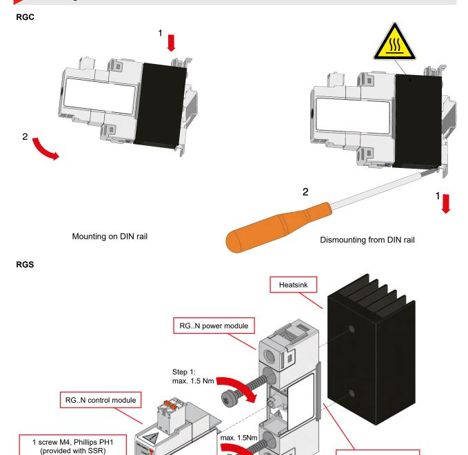
Step 1: Mount RG..N power module to Heatsink
