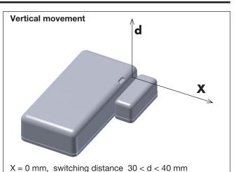
X = 10 mm, switching distance 25 < d < 35 mm X = 20 mm, switching distance 15 < d < 25 mm
