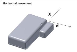
X = +/-5 mm, switching distance 20 mm < d < 30 mm X = 30 +/-5 mm, switching distance 7.5 mm < d < 15 mm
